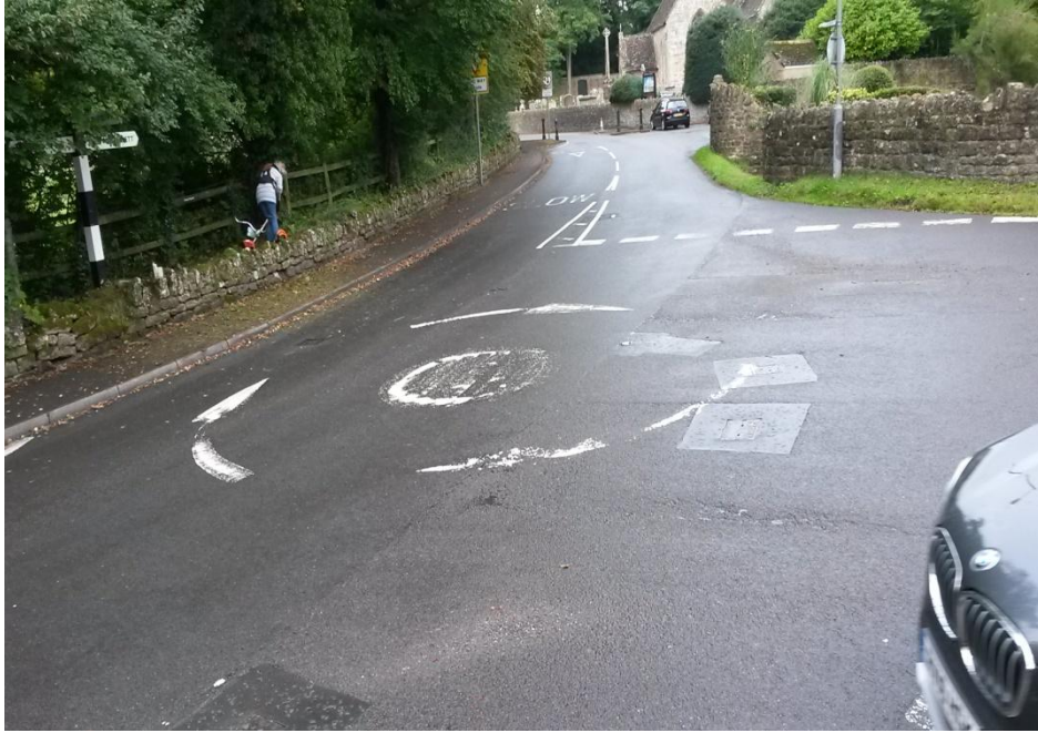
Photo 4-The painted mini roundabout at the junction of Church Place and The Street.
